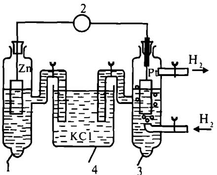
**12.4- rasm.** Metallning standart elektrod potensialini o'chash uchun galvanik zanjir:
